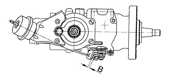
Connect up vacuum pump to pneumatic actuator.
